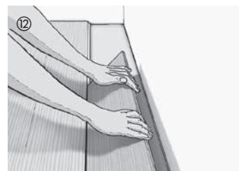
When the entire surface is finished the first two rows are removed again and laid without the protective film as described in points 8 and 9.
