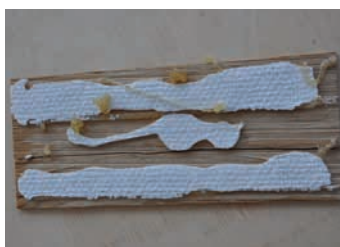
Adhesion test with a wall test sample
