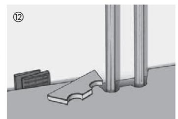
⑫ If radiator pipes protrude from the floor, drill or saw a cutout into the board (the size of the cutout depends on the radiator pipe and the required expansion space).
