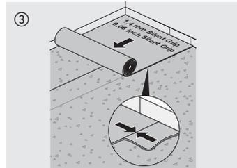
③ For sound insulation and to smooth out slight irregularities of the subfloor, unroll 1.4 mm thick Silent Grip underlay. Do not overlap. Our range of accessories also offers alternative insulation underlays. Asphalt-bitumen felt is not suitable for sound insulation.
