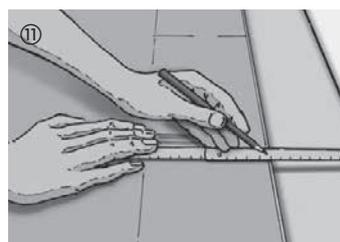
⑪ Cut to size and fit in the boards of the last row. Leave a gap of 7 to 10 mm between the boards and wall.
