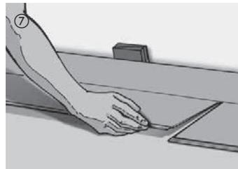
⑦ The next row is started with the leftover piece of the first row (short side offset of at least 50 cm, for tile format at least one-third of the element length). This considerably reduces waste. The rest of the installation is performed board-by-board. First, the boards are angled into the previous row along the long side by applying a small amount of force.
