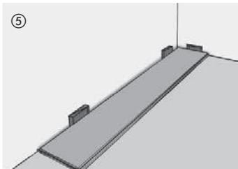
⑤ Starting in the right-hand corner of the room, align the boards of the first row with the tongue side parallel to the wall, and fix them in place with wall spacers as you proceed (always keep an expansion gap of 7–10 mm (3/8" - 1/2") around perimeter).
