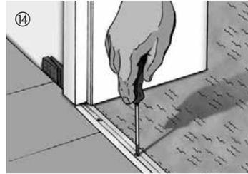
Leave an expansion space of approx. 5 mm between the board and the base of the moulding. As a rule, a fine saw must be used to cut a gap the thickness of a board in wooden door frames to allow the Design Floor floor to expand. Be sure to remove all distance spacers once all boards are laid. Fasten skirtings (with or without clip system) to the walls -- that's it.
